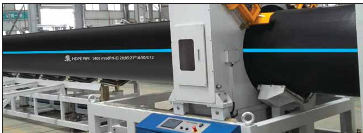
1400 mm RFL HDPE Pipe Production
